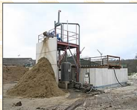
The earth-walled lagoon that once held up to 2500cu m of slurry now houses a 150cu m slurry reception tank, the DIY-built gantry supporting the FAN screw press separator and a bulk storage area for extracted fibre. Separated liquid is distributed from a 20,000cu m reservoir by irrigator or field applicator.
