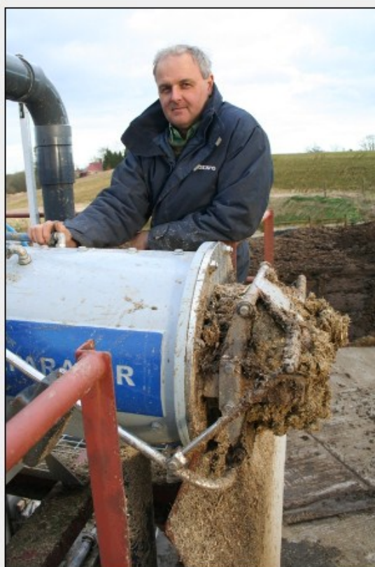
Neil Harrison with the FAN separator. Friction between the solids plug and cylindrical mouth-piece of the FAN separator, together with the adjustable weighted outlet flaps, create counter-pressure for forced dewatering.
