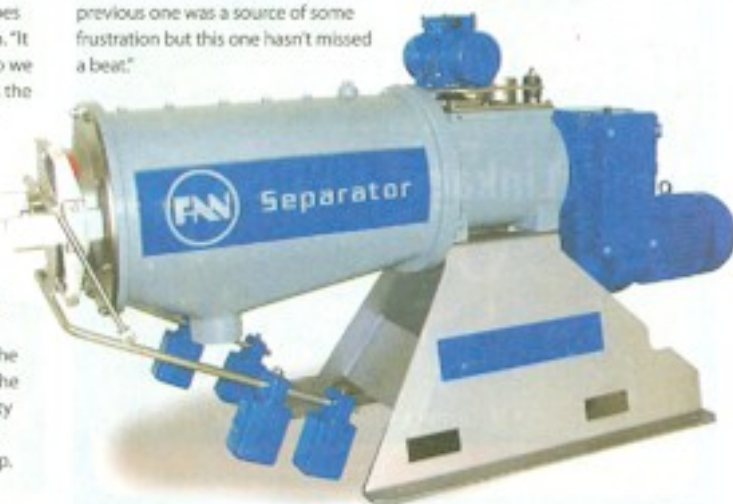
The Fan PSS 3.2-780 press screw separator has several patented features, including an oscillator that transmits pressure pulses into the inlet chamber to assist separation of sticky waste materials.
